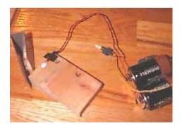
Here's the pieces about to be assembled. The light is layed in a channel I cut in the wood with a utility knife. You could also drill it (actually I drilled first, then enlarged it with the knife. Wires are just soldered onto the bulb. Lacking a soldering iron, I suppose you could try superglue, just try to keep some bare wire touching the bulb without glue. Note the 1/8" hole drilled in the aluminum cap (cover). This is placed directly over the bulb seen behind it on the wood.
