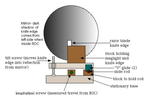
To perform the Foucault test or to adjust the Ronchi bands to appear where desired, the tilt screw is used to tip the entire top portion of the platform, as seen below:
